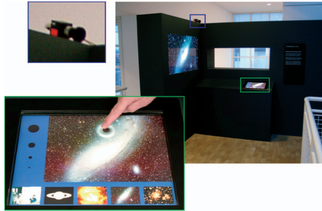
Fig. 8. Museum installation for the visualization of gravitational light bending. A black hole serves as a gravitational source and can be interactively controlled by direct manipulation on the touch panel. The background image can be chosen from a collection of stored astronomical pictures or from real-time camera input (top-left part of the image).
